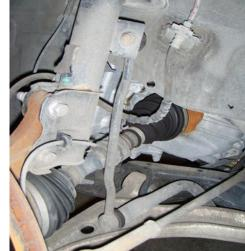
3. Install endlinks ball joint side up as shown.
