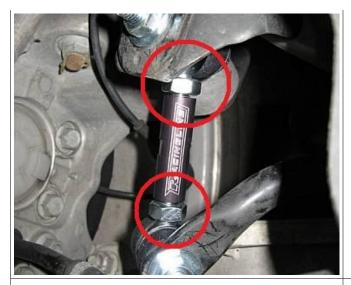
6. Tighten bushing/rod-end portions first. When secure, proceed to tighten rod-ends to the black turnbuckle, taking note that the left hand nuts will spin the opposite direction when tightening.
