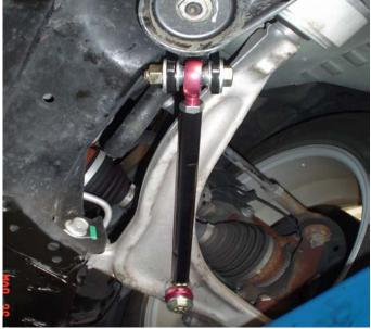
**5**.The above illustration shows the correct sequence of parts for the front assembly **(Top view)** --Control arm—bushing--washer-- nut-- nut.
