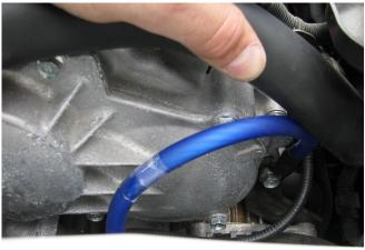
**11.**Wire#1- from passenger side engine mount (18mm bolt Image below))-to-alternator bracket (14mm socket). Be sure to leave enough slack in the wire to compensate for engine motion while driving, as the engine will rock back and forth.
