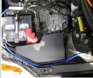
**8.** Wire#4-from rear cylinder head-to- existing threaded bolts at base of Driver strut tower
