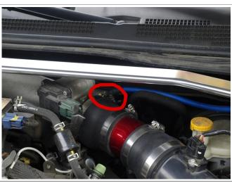
7. Wire #1 from throttle body to driver side strut tower
