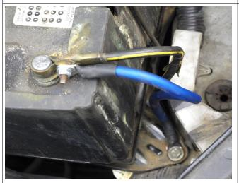
**9.** With all other wire now installed attach wire #1 to the battery tray and the negative terminal on the battery using supplied nut and washers.
