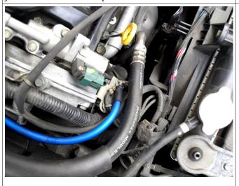
**8.** Wire #1 from existing ground on top of alternator to timing cover
