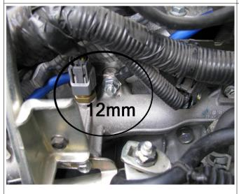
**4**. Wire #7 from transmission to front cylinder head, just above coolant line.
