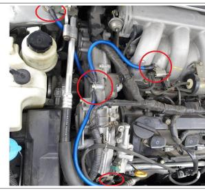
**9.** Wire #'s 1,1,1 to timing cover- Install using supplied bolt and washer. Wires #1 -to- passenger side strut tower and upper intake manifold.
