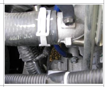
**3.** Wire #7 from trans bolt (pics 1 & 2. located just in front of starter and below coolant line) to side of cylinder head.
