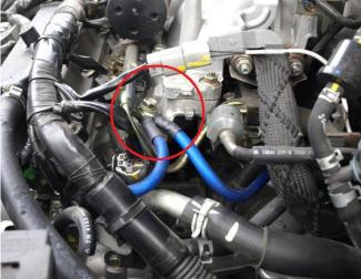
**5**. Wire #7 from front cylinder head ( step 4) to bolt located on lower intake manifold/fuel rail
