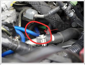
**6.** Wire #7 front lower IM (step 5) to rear cylinder head bolt just above coolant line. You will need a 12mm socket, u-joint-and small extension piece to reach this bolt.
