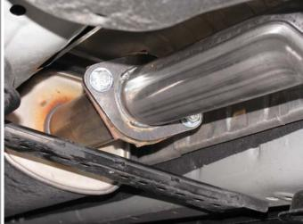
6. Use supplied 2x 10mm bolts tand associated harware to complete install of rear section.
